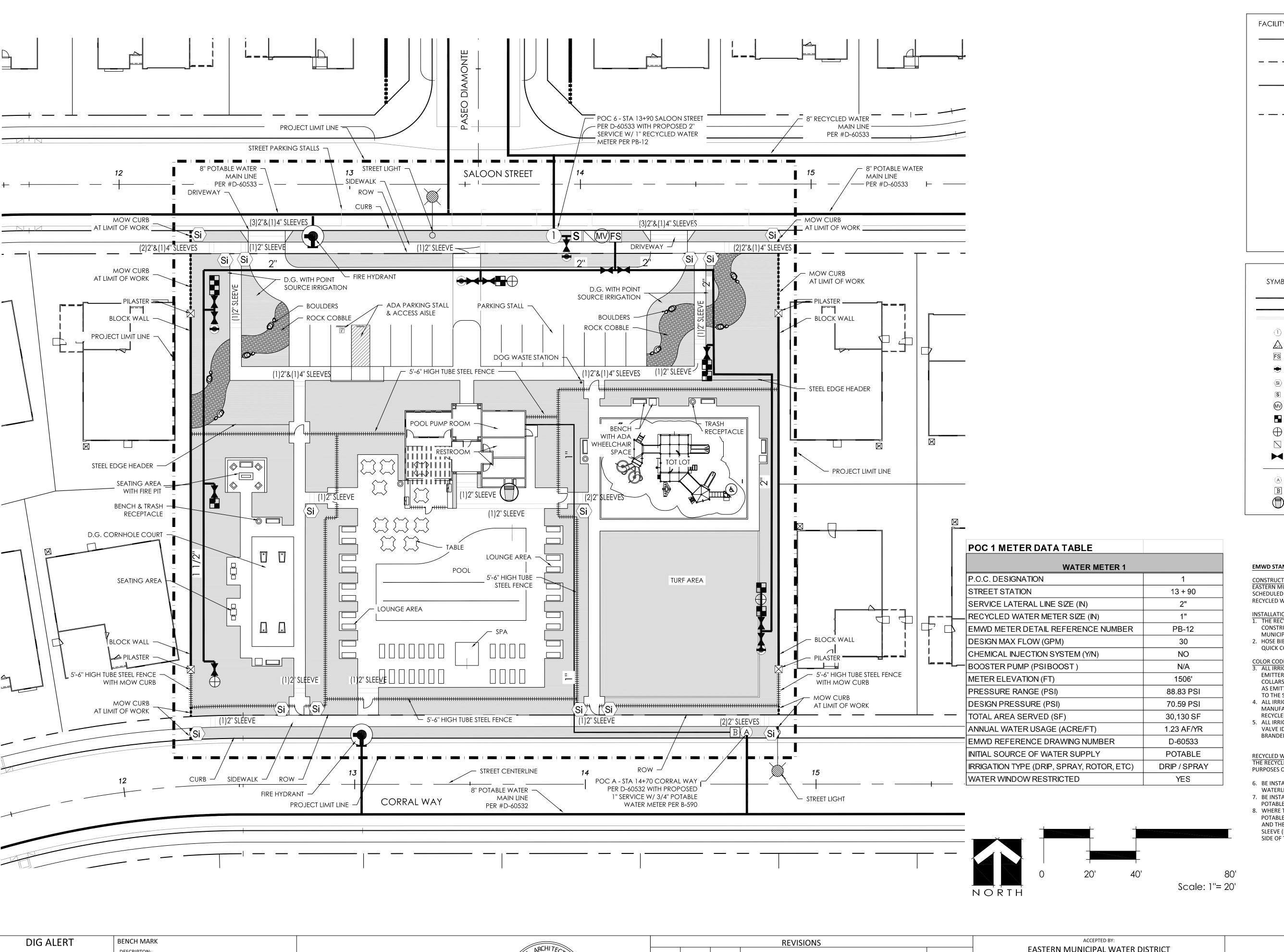
FACILITY WATER LEGEND PROPOSED POTABLE WATER MAINLINE (EMWD MAINTAINED) EXISTING POTABLE WATER MAINLINE (EMWD MAINTAINED) PROPOSED RECYCLED WATER MAINLINE (EMWD/ PRIVATE MAINTAINED) EXISTING RECYCLED WATER MAINLINE (EMWD MAINTAINED) BLOW OFF POTABLE (EMWD MAINTAINED) FIRE HYDRANT (EMWD MAINTAINED) BLOW OFF RECYCLED (EMWD MAINTAINED) STUB OUT RECYCLED WATER AIR VAC RECYCLED WATER AIR VAC POTABLE WATER
